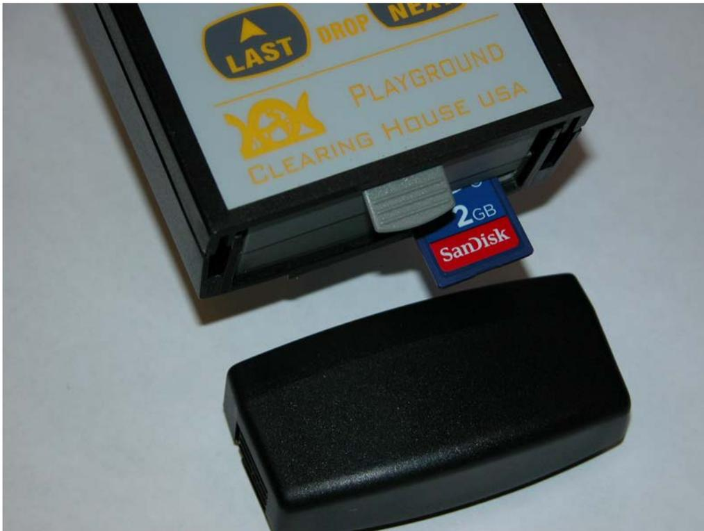
**Photo 2 – Battery Cover removed showing battery box and SD Memory Card**
